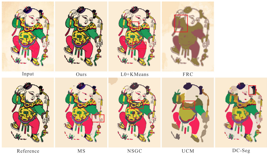
Fig. 16 Visual comparison of recomposition errors. The mean image of the man-made reference is shown, followed by those of results from L0+KMeans, FRC, MS, NSGC, UCM, DC-Seg and our method
