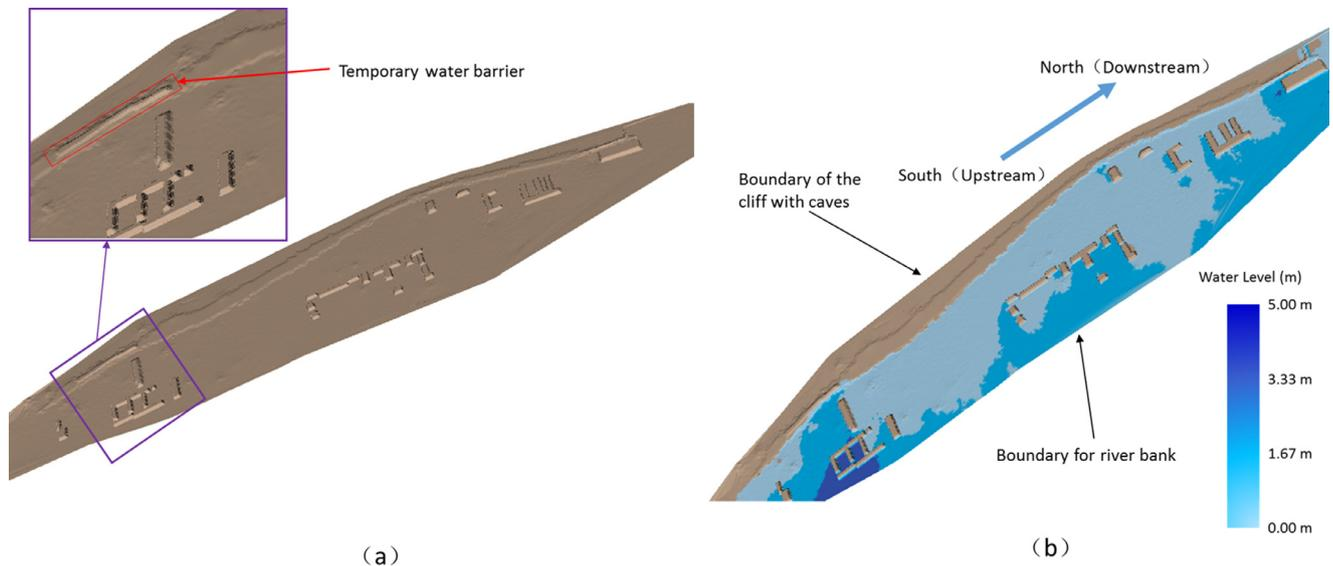
**Fig. 10.** Decision-making support to flood risk mitigation. (a) Temporary water barrier is added on the key position as a risk treatment measure. (b) Water level distribution on site after the 500-year frequency level flood that lasts for 3 h by implementing the risk treatment measure.
