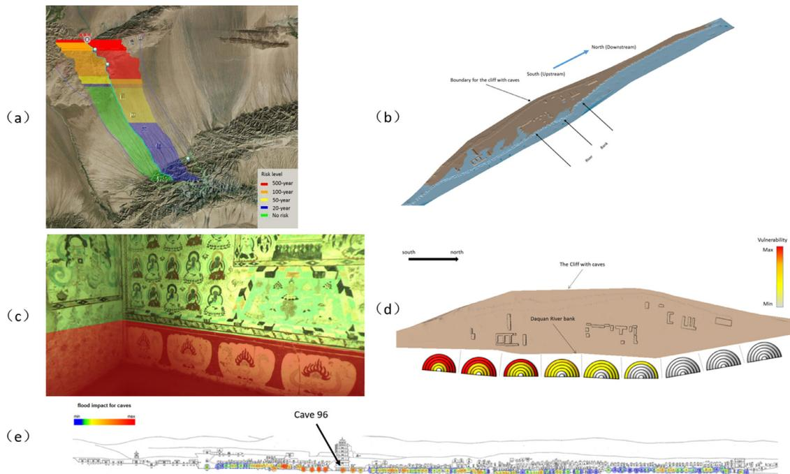
**Fig. 2.** Overview of all visualizations in the proposed visual analytics method. (a) Visualization of predicted flood peak flow based on GIS and aggregated bars. (b) Visualization of flood propagation based on 3D terrain model and color map. (c) Visualization of flood impacts to flood on cave level by panorama view. (d) Visualization of vulnerability based on concentric half rings plot. (e) Visualization of flood impacts on multi-cave level based on heat map.
