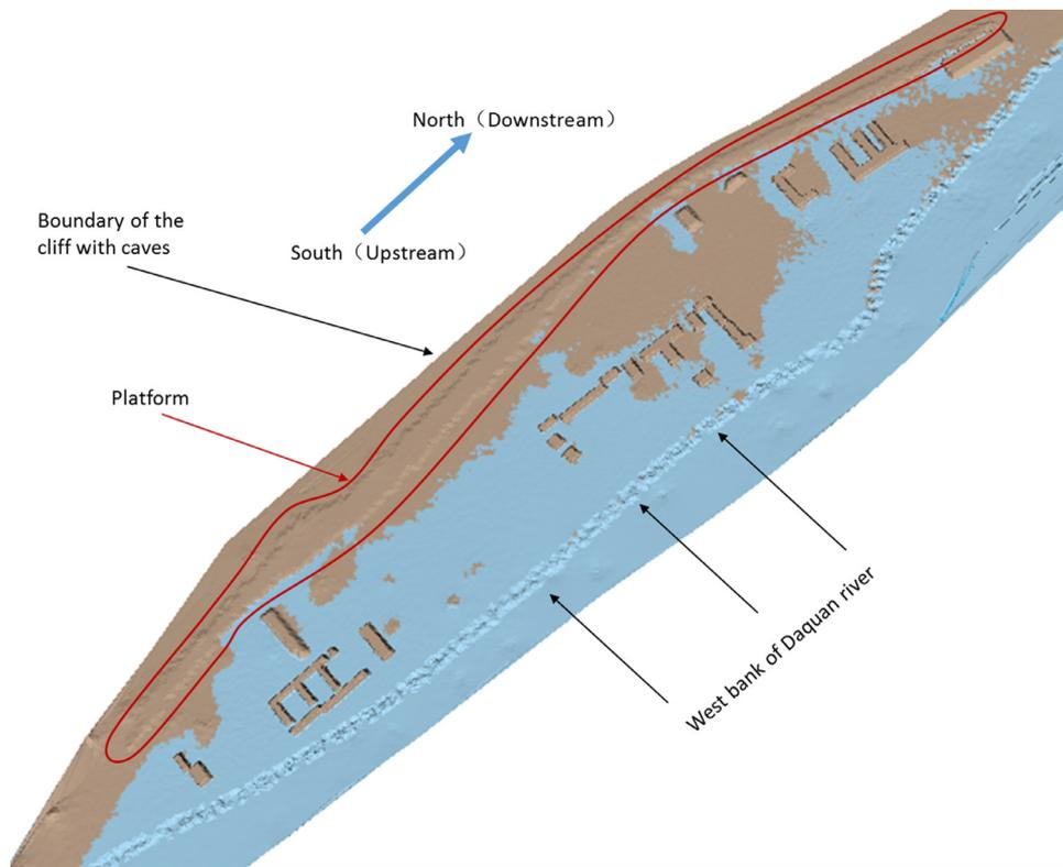
**Fig. 9.** Flood impact analysis of cultural relics. The Daquan River spills over its bank and water begins to flow into the site when flood exceeds the 100-year frequency level. However, the flood cannot affect the caves because the platform prevents the water from flowing in. The platform is marked by a red line in the figure.
