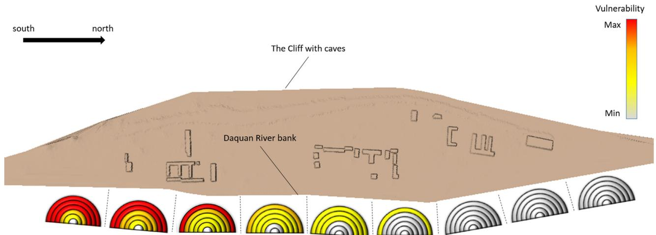
**Fig. 8.** Visualization of vulnerability to dike breaches. For a selected cultural relic (e.g., selected cave with mural paintings), the vulnerability to different breach positions and widths is visualized through the concentric half ring plot.
