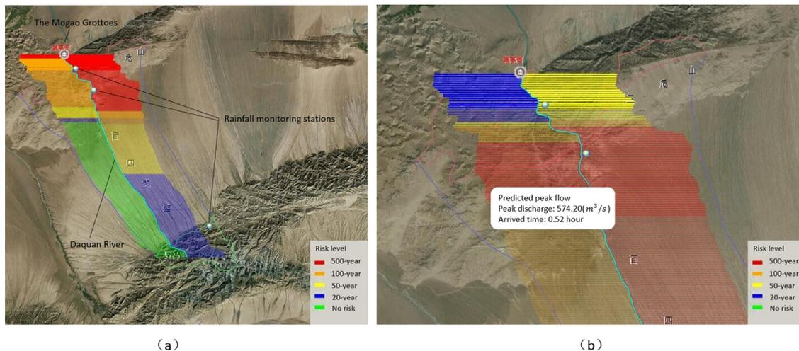
**Fig. 3.** Uncertainty-aware visualization of the temporal distribution of the predicted flood peak flow based on GIS on the basin scale. (a) Overview of the flood peak flow visualization. (b) Zoom-in view to show the horizontal aggregated bars.
