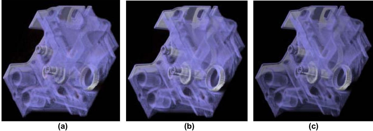
**Figure 1. Engine rendered with (a) DVR (b) distance weight boundary enhancement (c) original boundary enhancement and intensity depth cuing**
