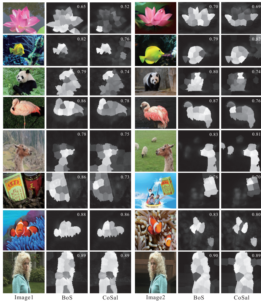
Fig. 7. Comparative co-saliency detection results: BoS vs. CoSal [12]. The F_\sigma measure is showed in the corner of each image, that is obtained by the weighted mean of precision and recall[12] using F_\sigma = \frac{(1+\sigma^2)\text{Pre}\cdot\text{Rec}}{\sigma^2\text{Pre}+\text{Rec}} , where \sigma^2 = 0.3 following the convention of co-saliency detection.
