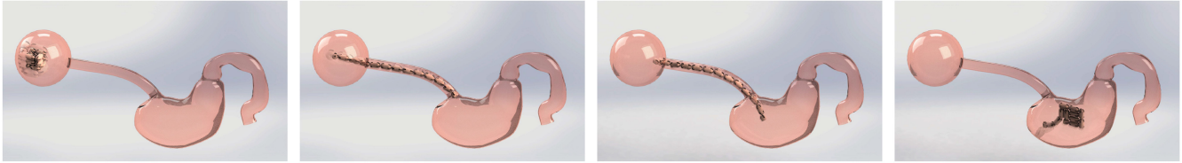
Fig. 20. Micro-robotic surgery using transforming structure generated by LineUp. A folded endoscopic device was placed into the mouth of a patient. One can unfold the device into a line configuration and then deliver it through the esophagus. After reaching the stomach, it can be folded into another endoscopic structure and is ready for operation. See also the accompanying video.
