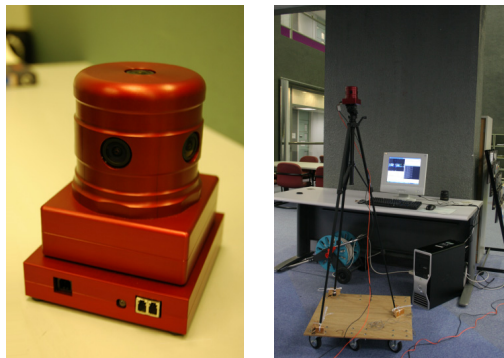
Fig. 8. Left: Ladybug2 camera. Right: the setup of our capture system: a PC, the Ladybug2 camera device, and a tripod attached on a movable platform.
