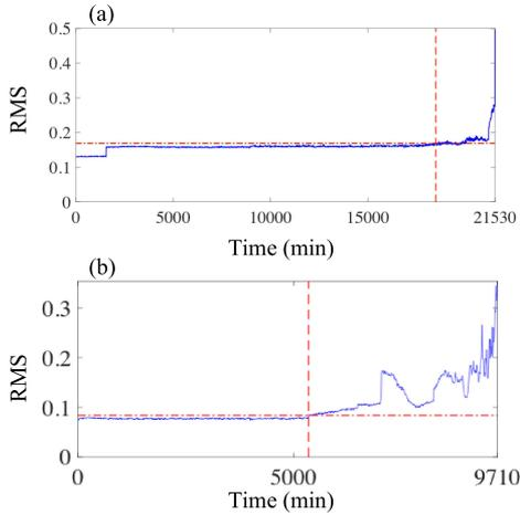
Fig. 5. IFP selection result of (a) dataset 1 and (b) dataset 2. The horizontal red line represents the rms threshold. The vertical red line represents the time point of IFP. The blue line represents the rms trend.
