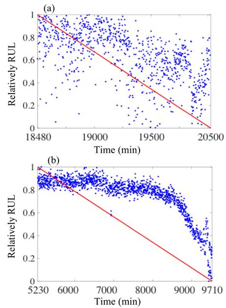
Fig. 10. SVR RUL prediction results of (a) dataset 1 and (b) dataset 2. The red line represents the real RUL. The blue points represent the predicted RUL.
