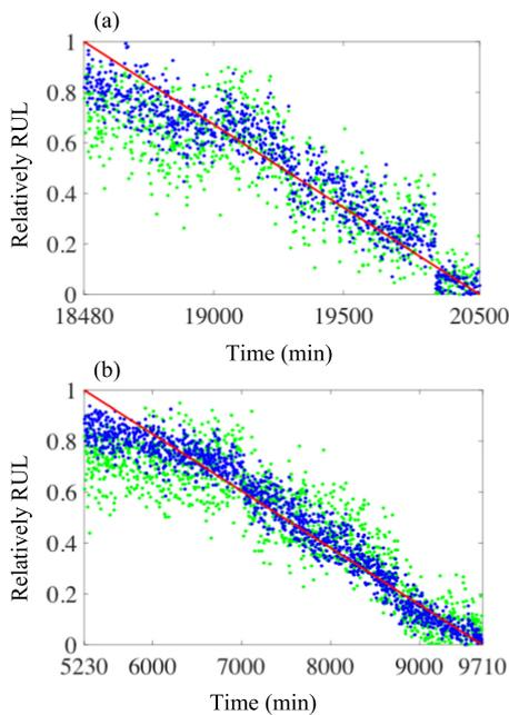
Fig. 9. RUL prediction results of (a) dataset 1 and (b) dataset 2. The red line represents the real RUL. The blue points represent the predicted RUL when  $\lambda = 0.25$ . The green points represent the predicted RUL when  $\lambda = 0$  that the network becomes a traditional CNN architecture.
