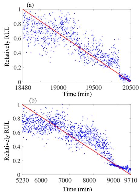
Fig. 11. HI-based RUL prediction results of (a) dataset 1 and (b) dataset 2. The red line represents the real RUL. The blue points represent the predicted RUL.
