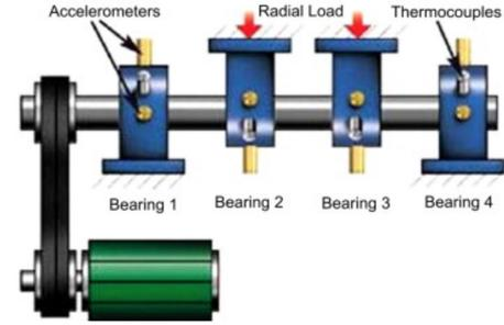
Fig. 4. Bearing test rig and sensor placement illustration.
