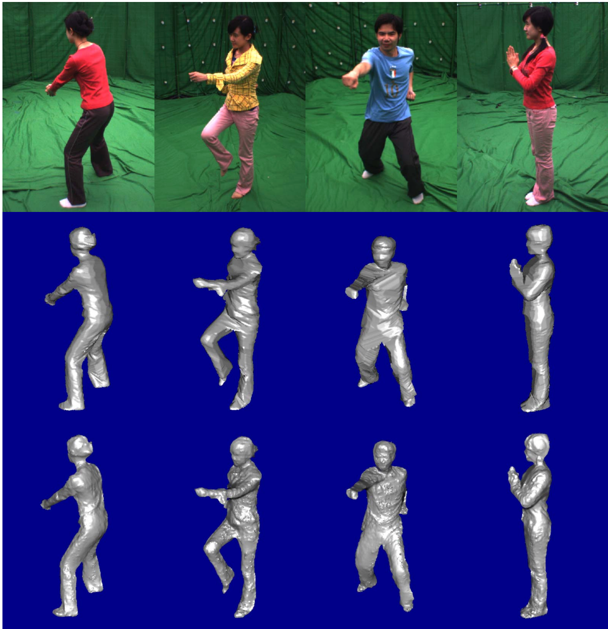
Fig. 7. Reconstructed depth maps of four datasets. Top row: four sample images of these datasets. Middle row: visual hull obtained from silhouettes. Bottom row: our reconstructed results in the separating step.
