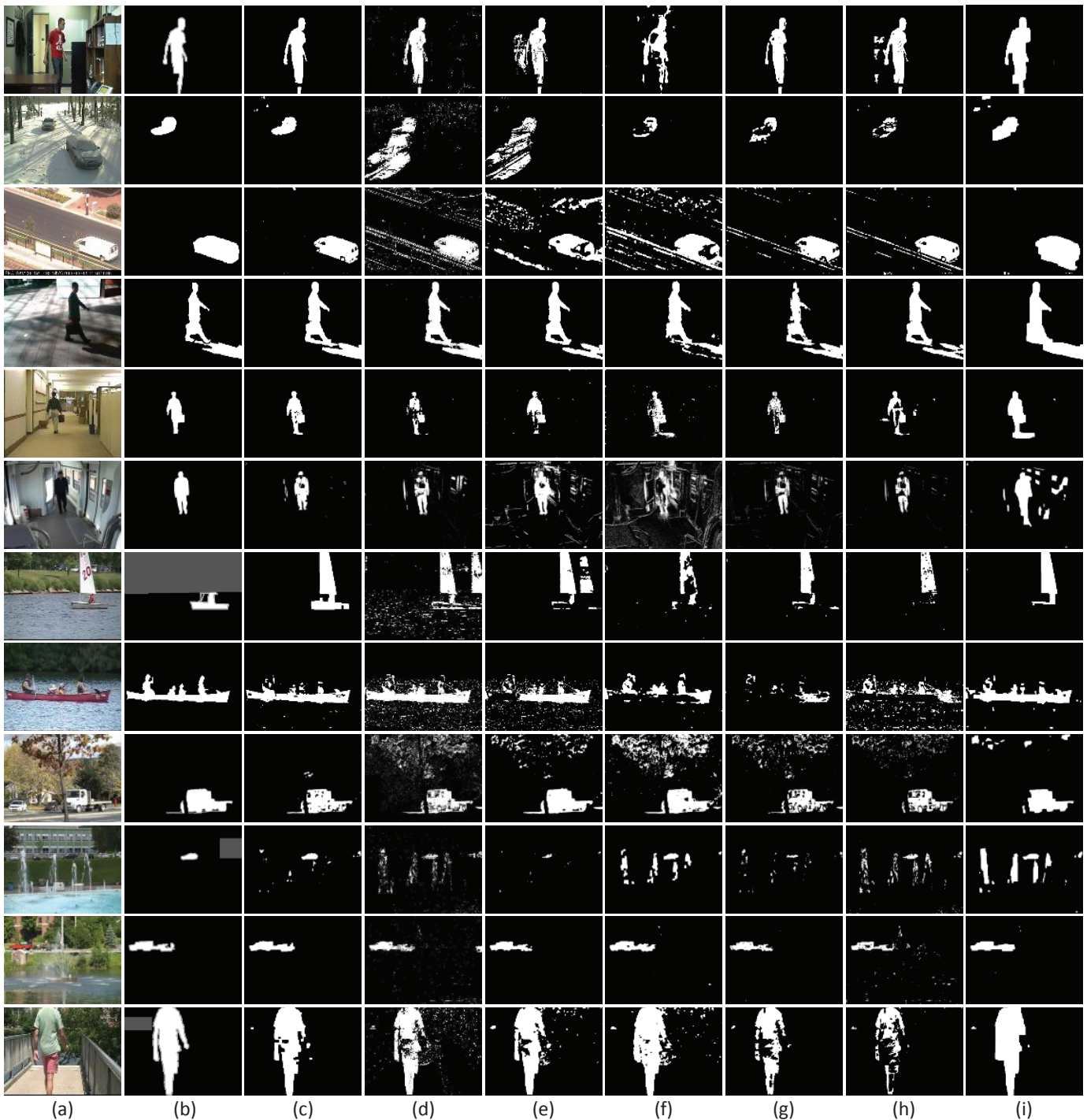
Fig. 9. Visual quality comparison for foreground detection on twelve video clips: (a) input image frame and (b) corresponding groundtruth binary foreground, (c) our MAMR model, (d) ViBe [21], (e)SOBS [25], (f)GMM [13], (g) FBM [28], (h) PCP [15], and (i) DECOLOR [9]. From top to bottom present the 656 th frame of Office , the 1936 th frame of Winter , the 816 th frame of Boulevard , the 481 th frame of Shade , the 56 th frame of Monitor , the 46 th frame of Train , the 7101 th frame of Boats , the 956 th frame of Canoe , the 1497 th frame of Fall , the 717 th frame of Fountain01 , the 741 th frame of Fountain02 , and the 2401 th frame of Overpass , respectively. The gray regions in the ground-truths provided by CDnet are excluded when making objective comparison.
