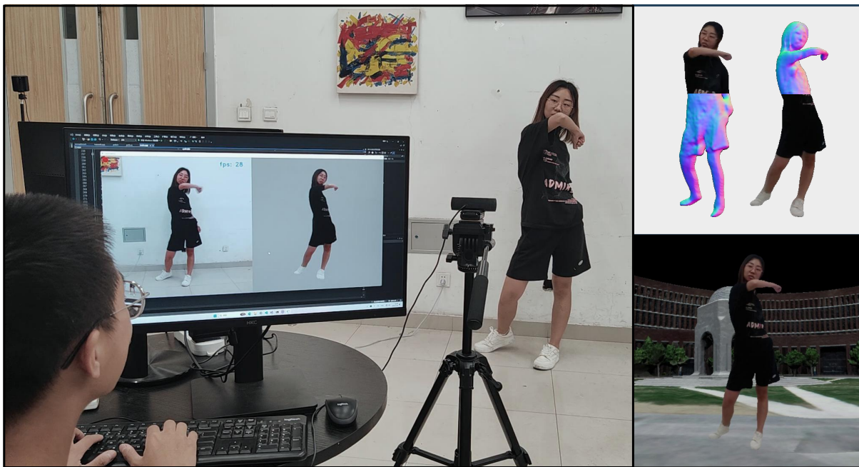
Figure 1: Our system achieves real-time high-quality 3D human reconstruction and rendering with a single RGB camera at 28+ FPS and exhibits an end-to-end latency of 75ms. It can be applied to 3D holographic displays and virtual reality environments.
