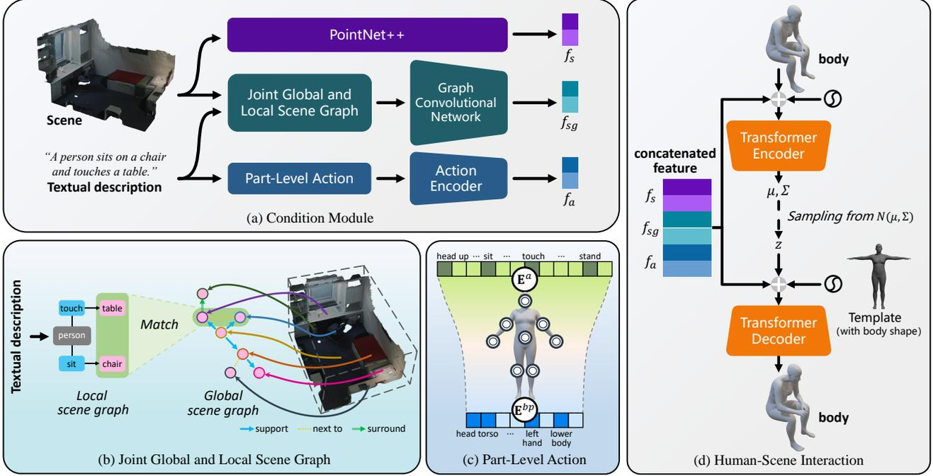
Figure 2: Overview of the proposed *Narrator* framework. Given a scene and a textual description, multi-modal features including scene features, scene graph features, and action features are extracted (a), where the latter two are reasoned through our Joint Global and Local Scene Graph (b) and Part-Level Action (c), respectively. These features are then concatenated as a joint conditional embedding and fed into the transformer-based cVAE framework for human-scene interaction (d).
