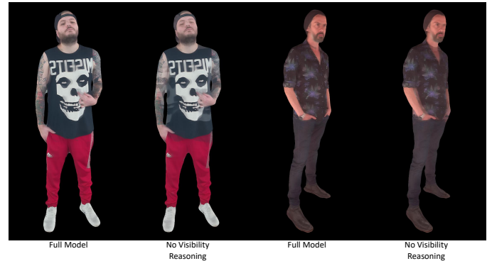
Fig. 8. Impact of pixel-wise visibility reasoning. If we warp all the source view pixels to the target view, the rendering results will suffer from severe occlusion problems caused by the wide camera baselines, resulting in blurring and artifacts.
