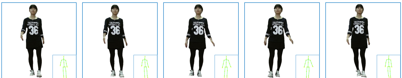
Fig. 8. Five frames of our created video for the actor without clenched fists. The inlays show the associated query skeleton used to create the target frame.
